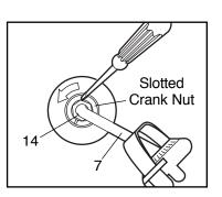
dard screwdriver in one of the slots in the slotted crank nut. Tap the screwdriver with a hammer to turn the slotted crank nut counterclockwise until the arms are no longer loose. **Do not overtighten the slotted crank nut.** When the slotted crank nut is properly tightened, tighten the Hex Crank Nuts.
